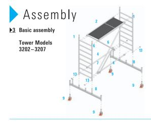
Insert the castors 9 into the mobile beam 8 and secure against falling out by fastening the bolts M  $12 \times 60$  and self-securing nuts through the holes provided. Insert the ladder frames 1 onto the mobile beam 8 and secure with spring clips 13. Clip the two diagonal braces 6 onto the ladder frames 1. Mount two guardrails 4 and one horizontal brace 7 onto the first rung of the ladder frame 1 from the bottom.
