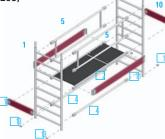
Insert ladder frames 1 and secure them with spring clips 13. Onto the 5th rung of the ladder frame from the top attach the access deck 2. Then build in the lateral protection with two double guardrails 5. After that mount two toe boards 1.8 m 11 between the ladder frames 1 and secure them by adding two end toe boards 0.75 m 10.
