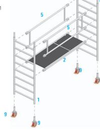
Insert the castors 9 into the ladder frames 1 and secure against falling out by fastening the bolts M 12x60 and self-securing nuts through the holes provided. Connect and brace both ladder frames 1 with two double guardrails 5. Clip the access deck 2 onto the 4th rung from the bottom. The snap-on claws of all parts are to be locked onto the ladder frames 1 from above.
